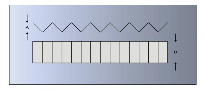
Sawtooth Ribbon Anodes are manufactured using Titanium which meets ASTM B265 Grade I, that has been coated with Mixed Metal Oxide (MMO) coating.
